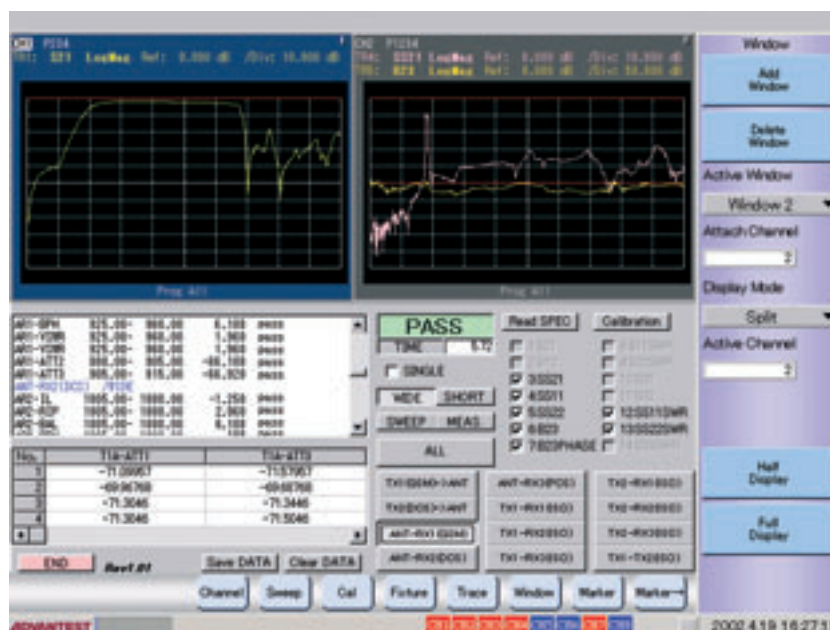
FIG 4 Analysis of antenna switching module of a mobile phone by means of an automatic test program.
