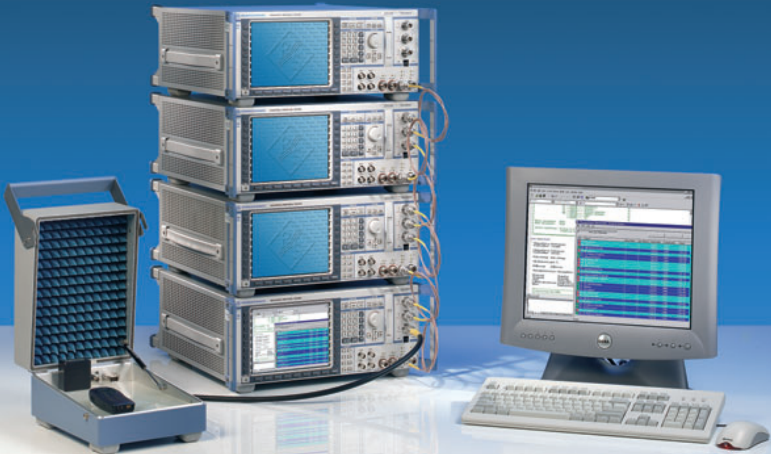
FIG 1 Cost-effective multicell system with a Universal Protocol Tester R&S CRTU-G and three R&S CRTU-S.
